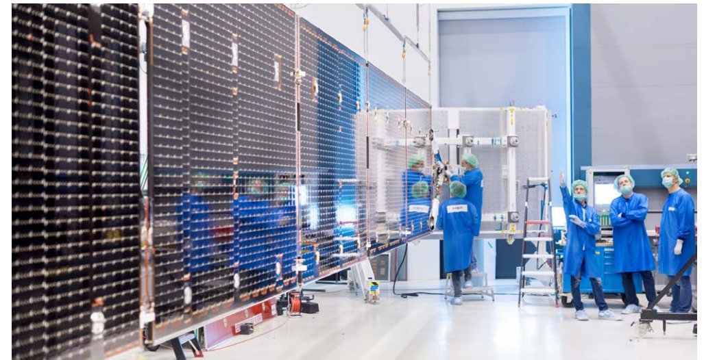
Dutch solar array for the European Service Module of the Artemis Moon mission of NASA and ESA ©Airbus Netherlands
